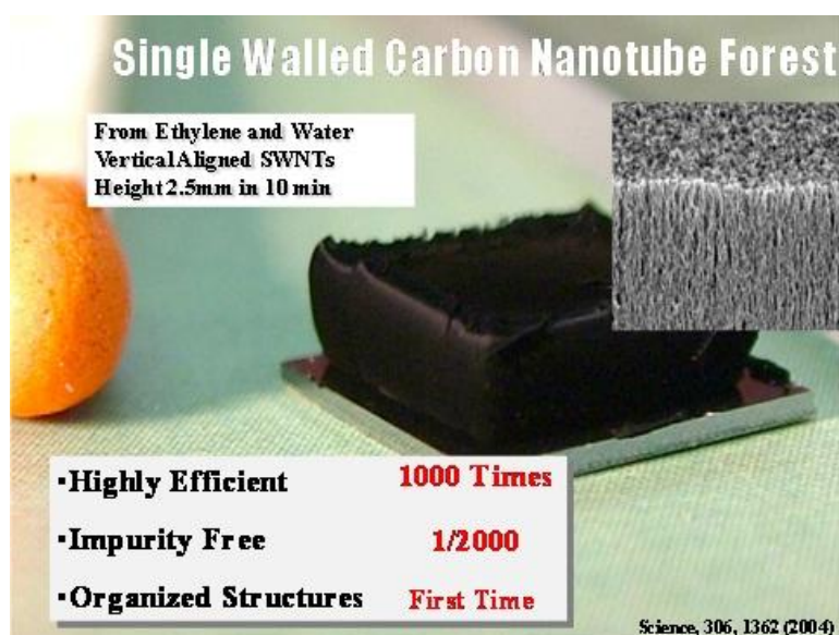
Figure 1. Single-walled carbon nanotube Forest (source: Dr Kenji Hata, AIST).
